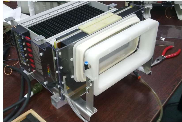
Photo of the assembled final T-GEM module with He buffer fitting.
